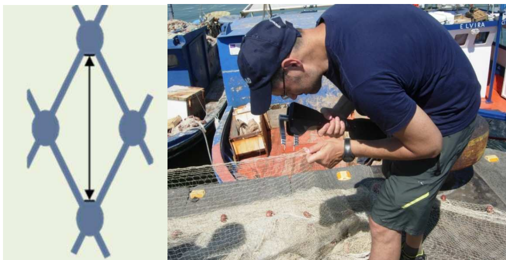
Figure 3.2.2 - Measurement of the mesh opening (left) of a “menaide” driftnet in the Catania fishing Harbour.
