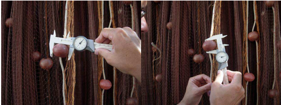
Figure 3.2.6 - Measurement of float's dimensions.
